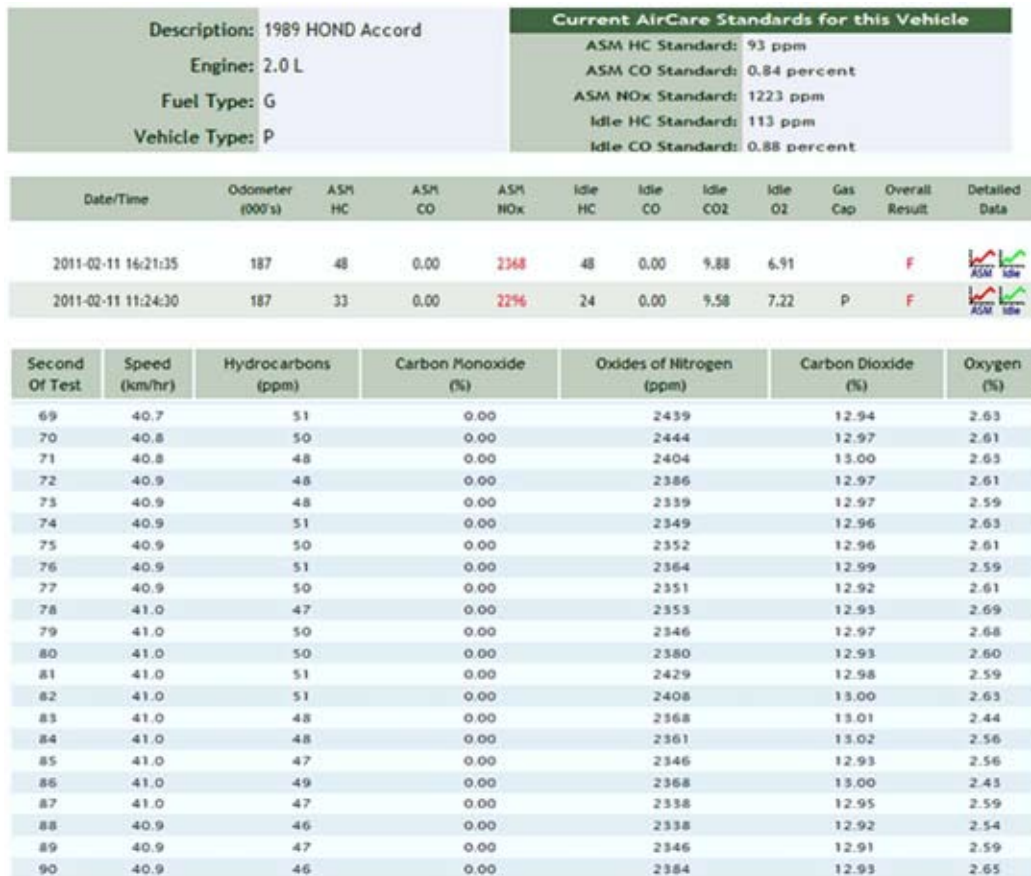
Figure 9: AirCare inspection history and last 20 seconds from RepairNet's Second-by-Second data for this ASM test
