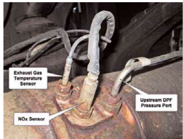
The 2011 Duramax SCR system is monitored using two NOx sensors. This photo shows the second sensor that is located between the SCR catalyst and the DPF.
