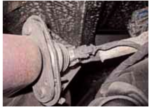
The DEF injector is located upstream from the SCR
