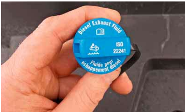
The DEF fill cap from a 2011 Duramax diesel specifies that the fluid must meet ISO 22241 standards.
